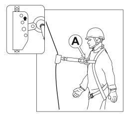
**ATTENTION**: Every time before using the equipment protecting against falls from height that employs the AC010 one needs to check if all the components are properly interconnected to one another and cooperate smoothly, as well as if they are compliant with compulsory standards:
