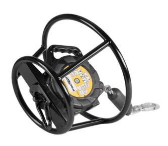
OS 050 is a steel rotating guard designed to work with CR 250HV retractable fall arrester. OS 050 is used to protect CR 250HV retractable fall arrester during horizontal operation during the movement of a user, e.g. along the roof edges, rotating together with retractable fall arrester.
